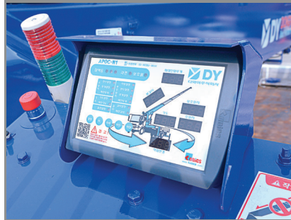
AML System for Safety Device
